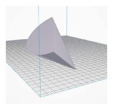
smoother surface is achieved with surfaces that are facing down, and a sharp surface is achieved with that surface facing up. Any feature such as a pin and clip that needs to hold a load should be positioned horizontally whenever feasible.
